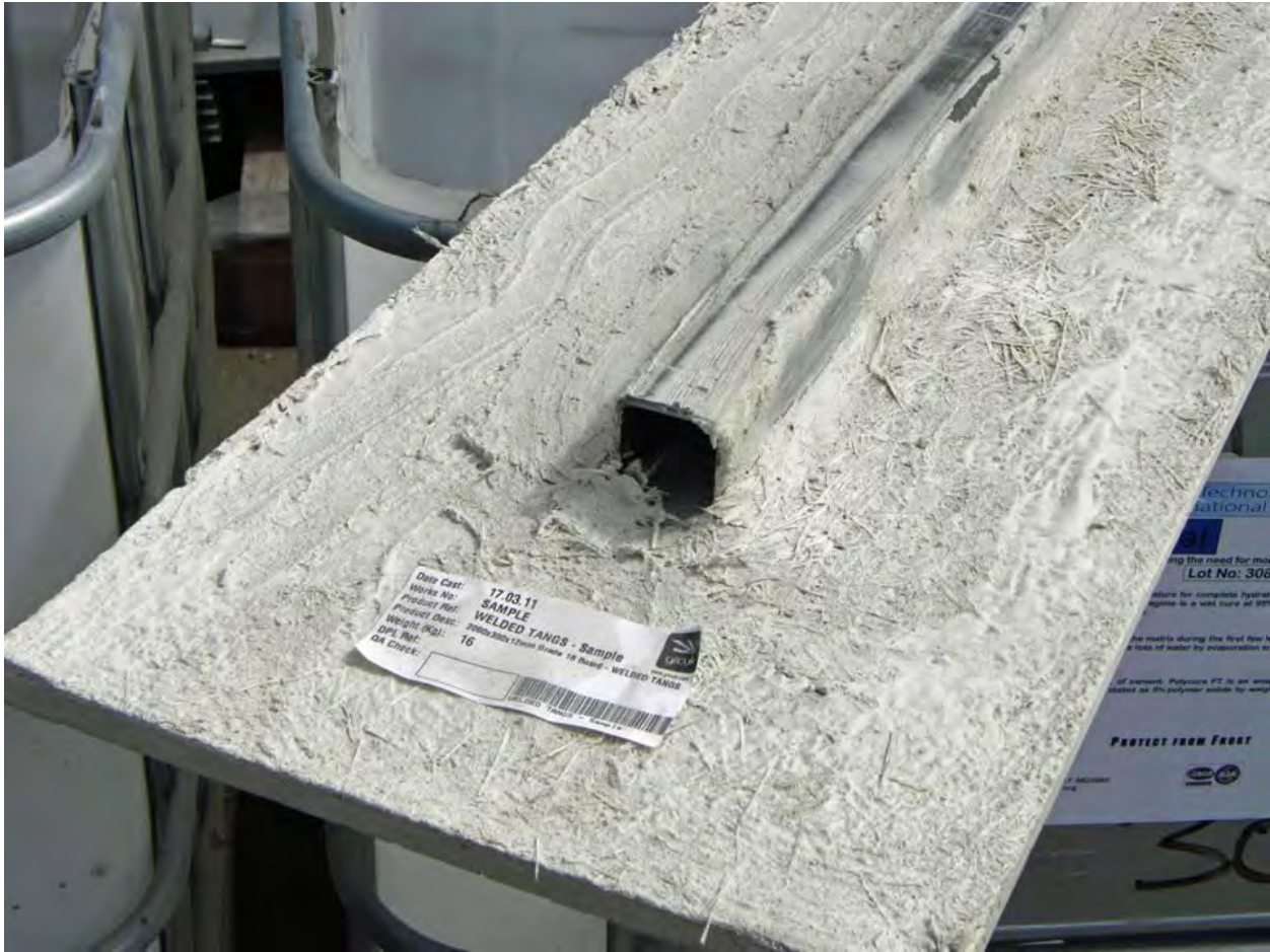
This photo shows a test sample using bent tangs to anchor the steel rib into the GRC facing.
