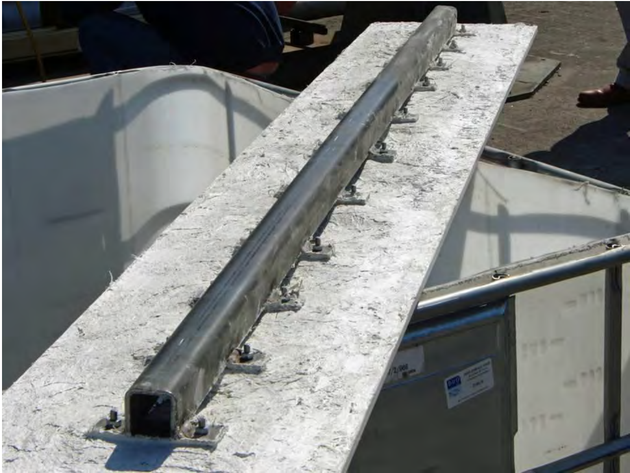
All the test samples had GRC facings 300mm in width. This slide shows a test specimen using bigHead fasteners to secure the steel rib.
